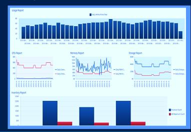
Usage metering and analytics are delivered by System Center 2012 R2 through Orchestrator as SPF web-services APIs, usage data is provided by Operations Manager and VMM. Windows Azure Pack surfaces the reports.
